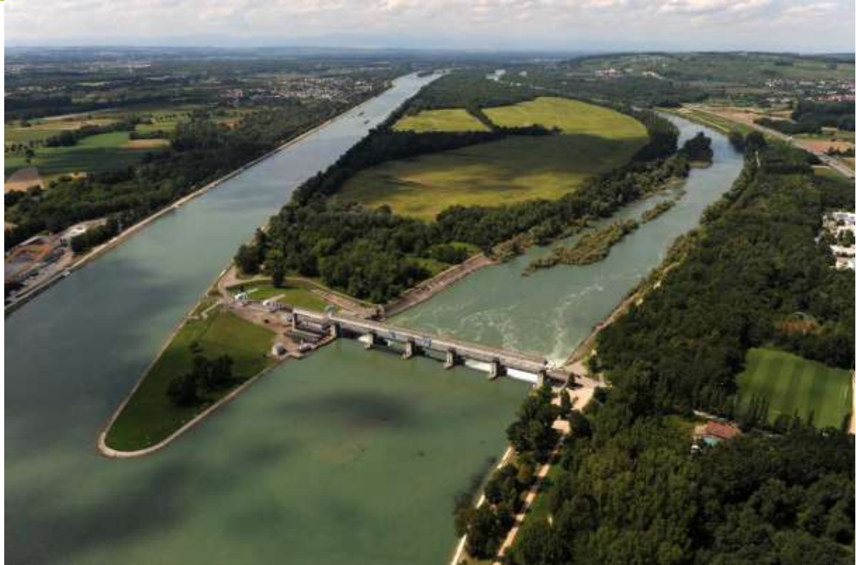
View of the situation of the Kembs power plant in the Upper Rhine valley in 2010. The stretch on the left side belongs to the Grand Canal of Alsace with the power plant at its far end. The river stretch behind the dam on the right is part of the Old Rhine (photo: EDF).
