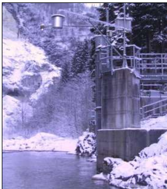
Figure 14: Hydrometric references; echo sounding automatic system and hydrometric rod for water level gauge
