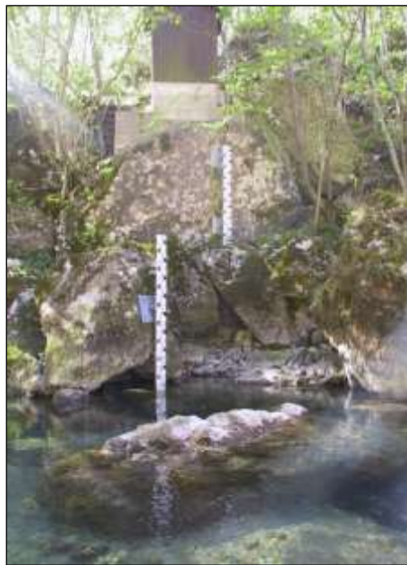
Figure 14: Hydrometric references; echo sounding automatic system and hydrometric rod for water level gauge
