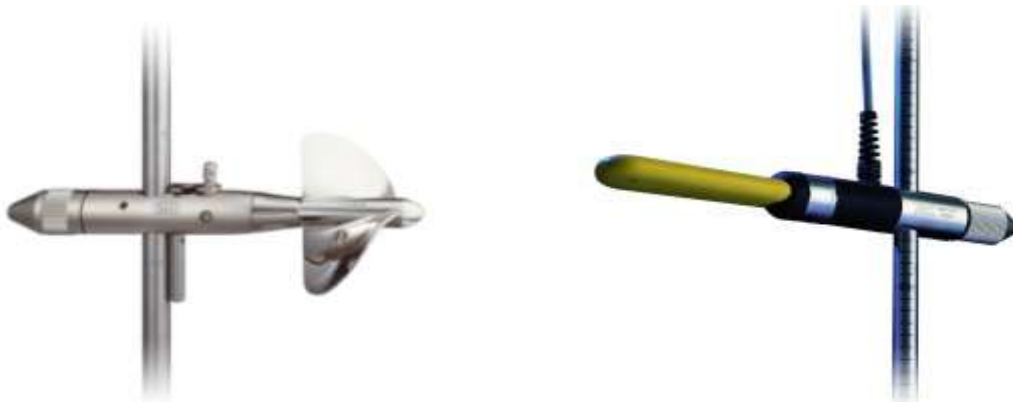
Figure 7: Current meters; classic and electromagnetic (ECM, Nautilus C2000) ones
