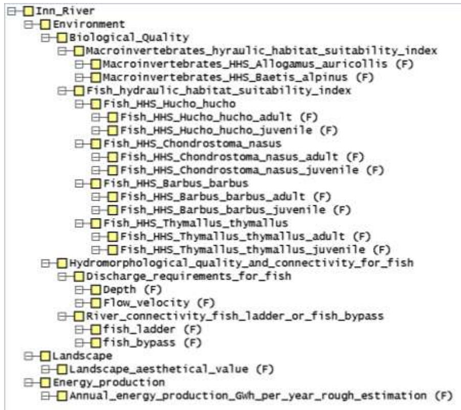
Image 8: SESAMO decision tree for the Inn meander and the HP plant Kirchbichl.
