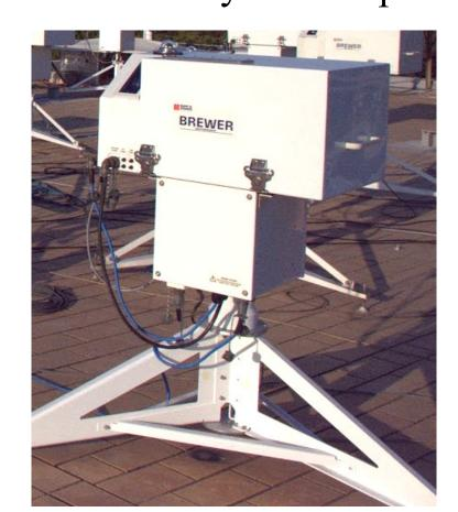
Three different Brewer models are in operation in EUBREWNET, all of which perform measurements at five wavelengths between 306 and 320 nm as part of their standard ozone measurement programs. Brewer instruments are reliable and stable, and are often calibrated just once every 2 years at international intercomparison campaigns.
