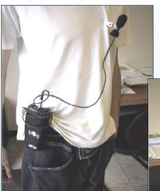
dosimeters used in order to allow the execution of the measurements hidden in order to render the operator undistinguishable from the other customers
